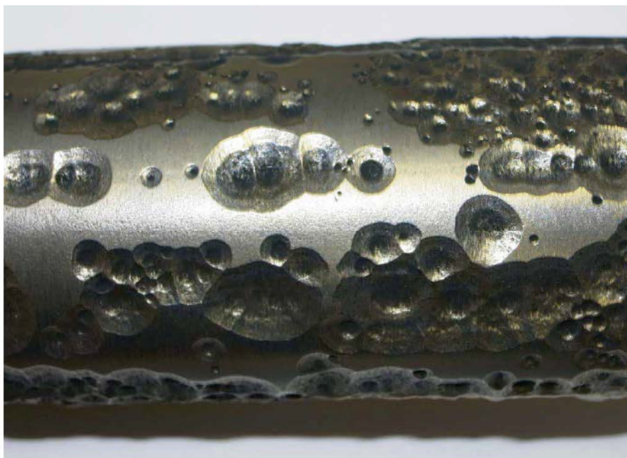
Fig. 1: Alloy 601 showing metal dusting pits.
